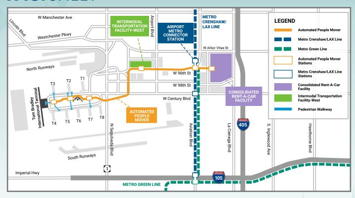
The APM will deliver passengers between LAX and new offsite parking, car rental, and transit facilities. The APM is one component of the larger LAMP. The LAMP consists of five major components: the APM, the Consolidated Rent-A-Car (ConRAC) Facility, Intermodal Transportation Facility-West (ITF-West), connection to Metro via the future Airport Metro Connector (AMC) Station, and roadway improvements throughout the LAX area.
